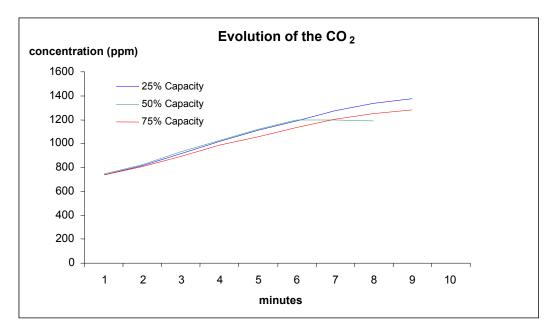
Pic. 3. CO<sub>2</sub> rate evolution with equipment turned on during combustion.
