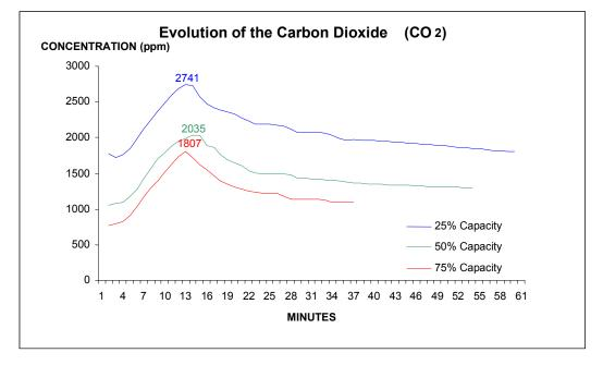
Pic. 4. CO<sub>2</sub> rate evolution with equipment turned off during combustion
