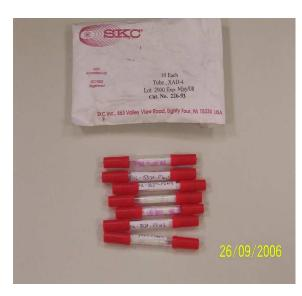
Fig 4. XAD-4 adsorbents, 80/40 mg
